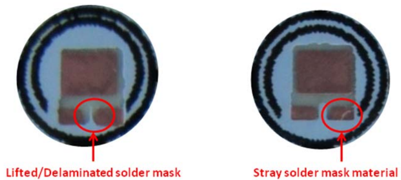
Figure 33. Examples of poor PCB workmanship which may adversely impact the solder joint between the PCB and the LUXEON emitter.
