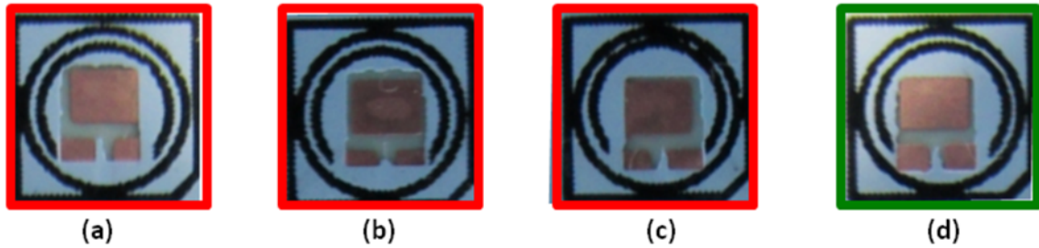
Figure 32. During PCB manufacturing poor positional control of the solder mask layer with respect to the top metallization layer can impact the actual pad dimensions on the PCB. The four pictures in this example were all taken from the same physical 4-up PCB. The anode and cathode dimensions for positions (a) – (c) on this PCB are smaller than originally designed. Only the pad dimensions for position (d) were in specification.
