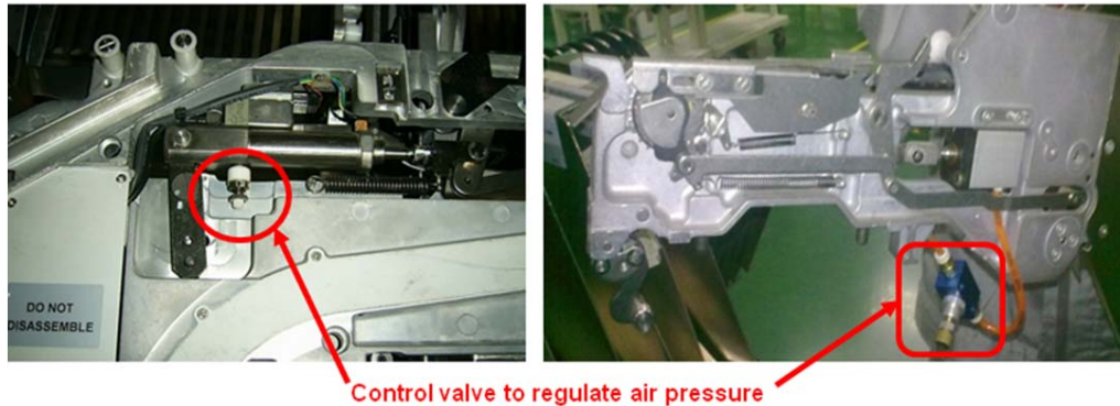
Figure 28. Pneumatic feeder with integrated air pressure control valve (left) and pneumatic feeder with air pressure control valve installed afterwards (right).
