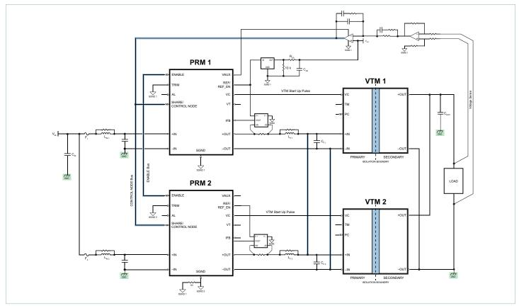
Figure 39 — Non-Isolated Remote Sense Array Example
