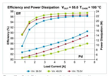
**Figure 12** — Total efficiency and power dissipation vs.  $V_{IN}$  and  $I_{OUT}$  = 55.0 V,  $T_{CASE}$  = 100°C
