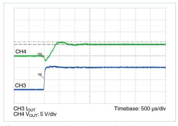
**Figure 35** — PRM Example 10% to 100% Load Transient Response, Adaptive Loop Load Line Enabled, V<sub>AL</sub> = 1.20 V
