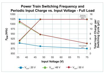
**Figure 14** — Typical Power Train Switching Frequency and Periodic Input Charge vs. V<sub>IN</sub>, V<sub>OUT</sub>; I<sub>OUT</sub> = 8.33 A
