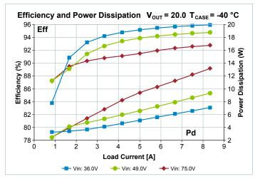
**Figure 4** — Total efficiency and power dissipation vs.  $V_{IN}$  and  $I_{OUT}$  = 20.0 V,  $T_{CASE}$  = -40°C
