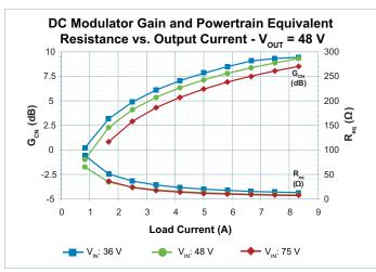
Figure 19 — Powertrain Characteristics vs.  $I_{OUT}$ ,  $V_{IN}$  Resistive Load,  $V_{OUT} = 48.0 \text{ V}$
