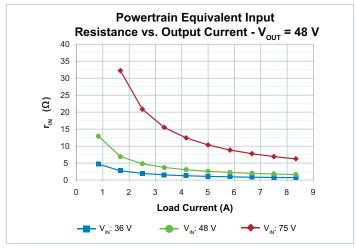
**Figure 22** — Magnitude of powertrain dynamic input impedance vs.  $I_{OUT_i}$  $V_{IN_i}$   $V_{OUT} = 48.0 \text{ V}$
