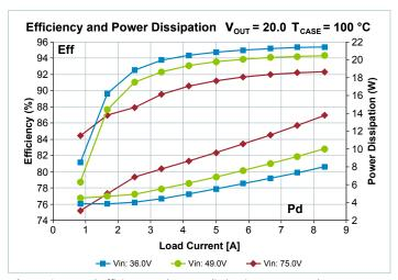
**Figure 6** — Total efficiency and power dissipation vs.  $V_{IN}$  and  $I_{OUT}$  = 20.0 V,  $T_{CASE} = 100^{\circ}C$
