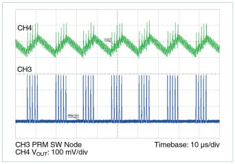
**Figure 41** — Light load burst mode of operation
