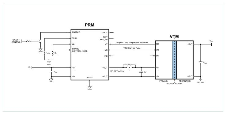
Typical Application: PRM48Ay480x400A00 + VTM Adaptive Loop Configuration
