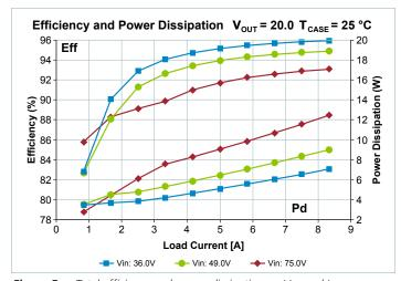
**Figure 5** — Total efficiency and power dissipation vs.  $V_{IN}$  and  $I_{OUT}$  = 20.0 V,  $T_{CASE} = 25^{\circ}\text{C}$
