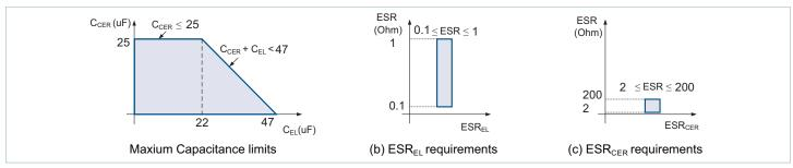
Figure 32 — Output Capacitance Limits
