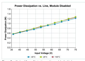
**Figure 3** — No Load Power Dissipation vs.  $V_{IN}$ , module disabled - Enable = Low
