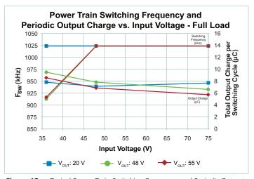
**Figure 15** — Typical Power Train Switching Frequency and Periodic Output Charge vs.  $V_{IN_r}$   $V_{OUT}$ ;  $I_{OUT} = 8.33$  A
