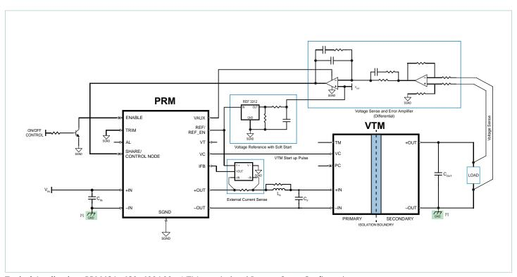
Typical Application: PRM48Ay480x400A00 + VTM, non-isolated Remote Sense Configuration
