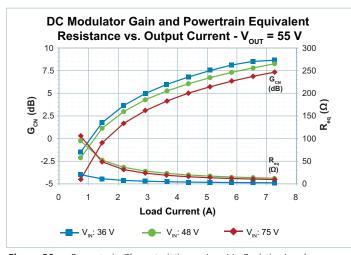
Figure 20 — Powertrain Characteristics vs.  $I_{OUT}$   $V_{IN}$  Resistive Load,  $V_{OUT} = 55.0 \text{ V}$
