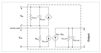
Figure 24 — PRM48Ay480x400A00 AC small signal model
