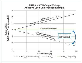
Figure 27 — Adaptive Loop Compensation Illustration
