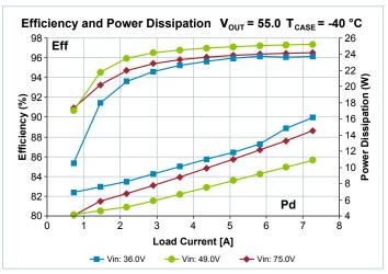
**Figure 10** — Total efficiency and power dissipation vs.  $V_{IN}$  and  $I_{OUT}$  = 55.0 V,  $T_{CASE}$  = -40°C
