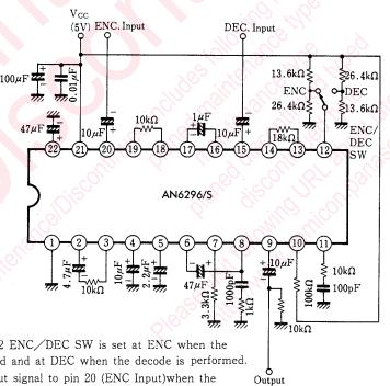
\*1 Set the pin 12 ENC/DEC SW is set at ENC when the encode is performed and at DEC when the decode is performed.
