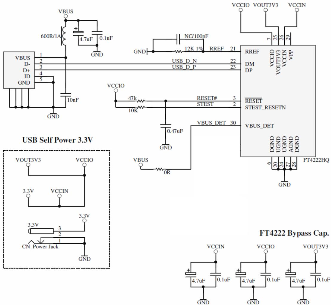
Figure 7.3 Self Powered Configuration with 3.3V Source Input
