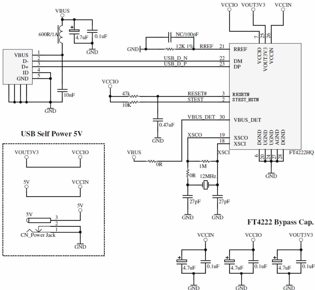
**Figure 7.2 Self Powered Configuration with 5V Source Input**
