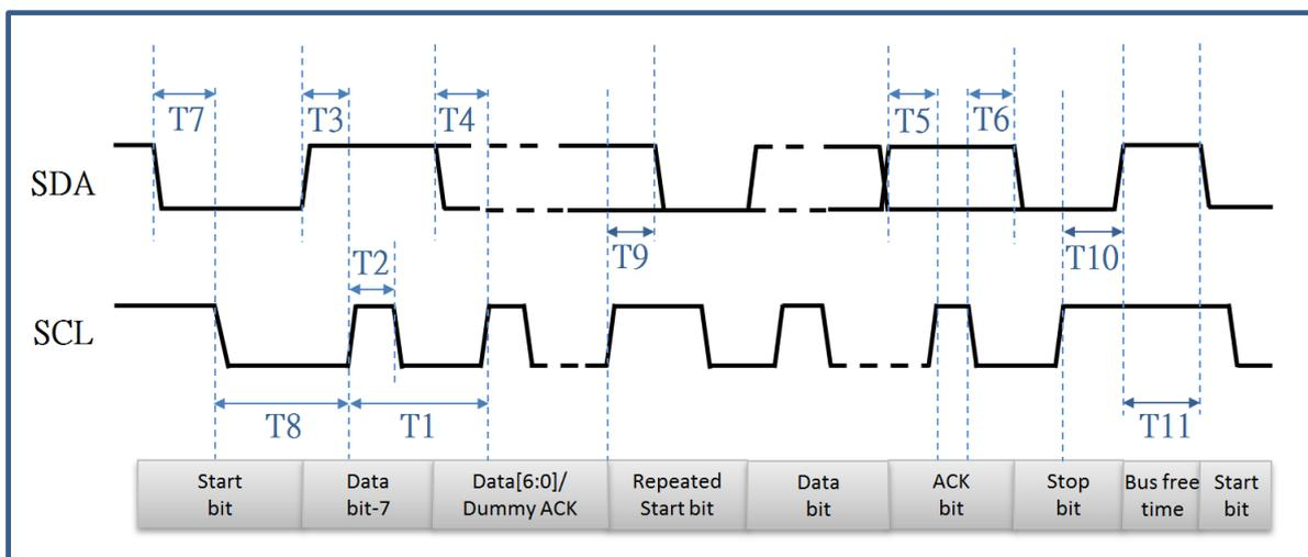
**Figure 5.7 I<sup>2</sup>C Bus Timing**
