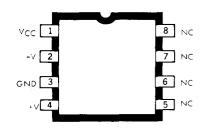
The UGN-3600M and UGN-3601M are intended for use as an empirical design aid or as a production test vehicle. Each device consists of the Hall generator only with connections brought out on pins 2 and 4. Type UGN-3600M is supplied with a calibration chart for monitoring magnetic field intensity without the use of a gauss meter. Type UGN-3601M is supplied without the calibration chart.
