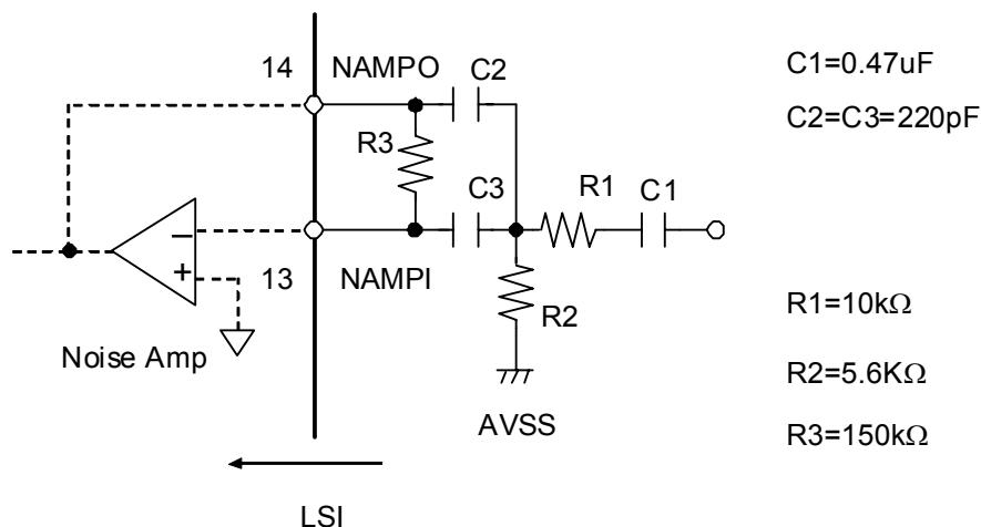
$$(1) \quad f_0 = \frac{1}{2\pi\sqrt{R_3(R_1//R_2)C^2}}$$
