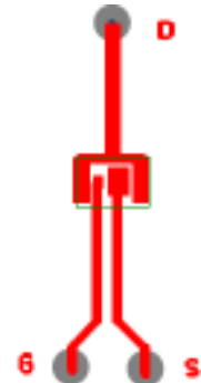
⑧ Mounted on minimum footprint full size board with metalized back and with small clip heatsink (still air)
