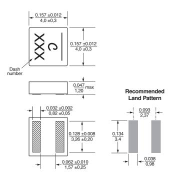
Dimensions are in  $\frac{\text{inches}}{\text{mm}}$
