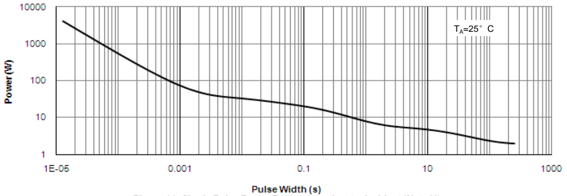
Figure 14: Single Pulse Power Rating Junction-to-Ambient (Note H)
