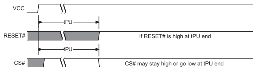
Figure 6.5 Reset High at the End of POR
