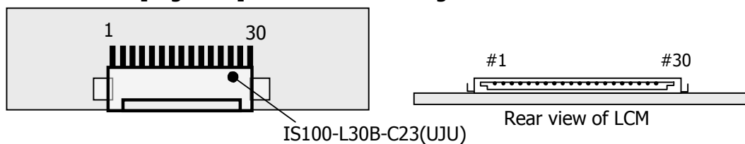
[ Figure 4 ] User Connector diagram
