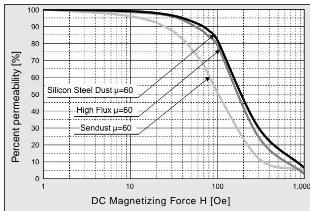
**◆D.C. bias of Dust core (2)**
