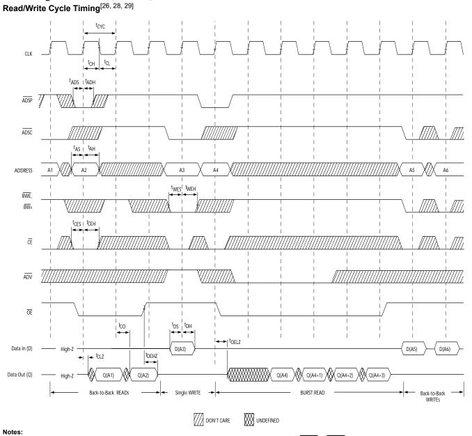
28. The data bus (Q) remains in high-Z following a Write cycle, unless a new read access is initiated by ADSP or ADSC. 29. GW is HIGH.
