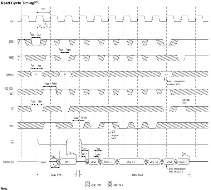
26. On this diagram, when  $\overline{CE}$  is LOW:  $\overline{CE}_1$  is LOW,  $CE_2$  is HIGH and  $\overline{CE}_3$  is LOW. When  $\overline{CE}$  is HIGH:  $\overline{CE}_1$  is HIGH or  $CE_2$  is LOW or  $\overline{CE}_3$  is HIGH.
