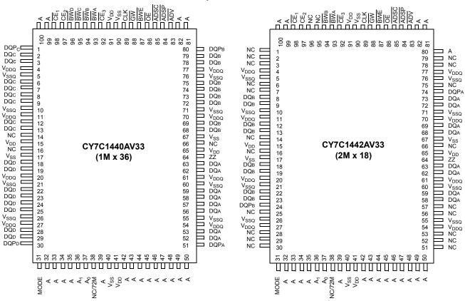
**100-pin TQFP Pinout**
