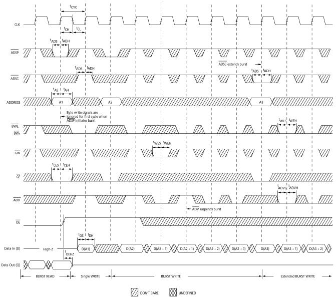
Note: 27. Full width write can be initiated by either  $\overline{GW}$  LOW; or by  $\overline{GW}$  HIGH,  $\overline{BWE}$  LOW and  $\overline{BW}_X$  LOW.
