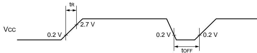
If you change the power supply voltage too rapidly, a power-on reset may occur. We recommend that you start up smoothly by restraining voltages when changing the power supply voltage during operation, as shown in the figure below. Perform while not using the PLL clock. However, if voltage drops are within 1 V/s, you can operate while using the PLL clock.
