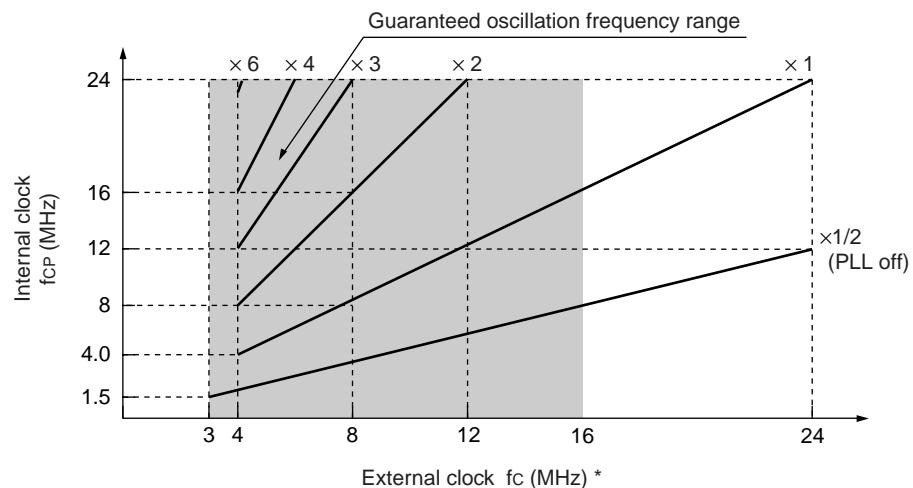
\* : When using the oscillation circuit, the maximum oscillation clock frequency is 16 MHz.
