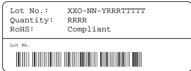
Figure 20: First label on reel: XX = Sensor Type (25 for SHT25), O = Output mode (0 = Digital), NN = Chip Version, Y = last digit of year, RRR = number of sensors on reel divided by 10 (200 for 2000 units), TTTTT = Traceability Code.
