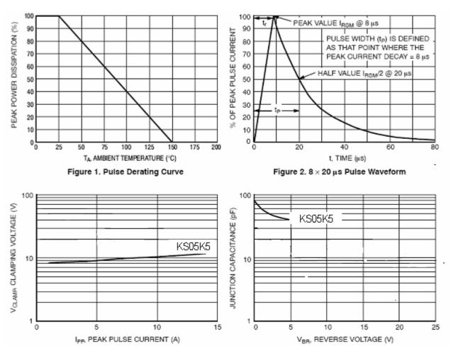
Figure 3. Clamping Voltage vs Peak Pulse Current
