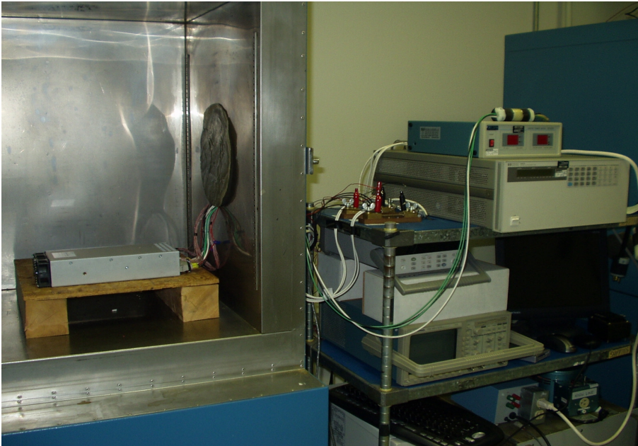
Typical thermal survey and HALT setup.
