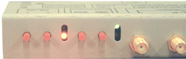
Figure 3: N4915A-005 front view with status LEDs
