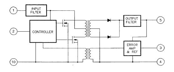
FIGURE 3. Block diagram.
