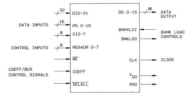
FIGURE 2. Block and logic diagrams.
