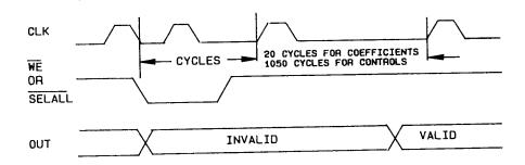
FIGURE 3. Timing waveforms - Continued.
