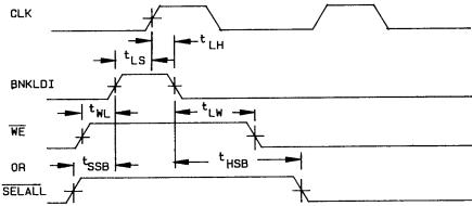
Synchronous Loading of Master and  $\underline{\text{Syn}}$ chronous Transfer to Slave Section with  $\underline{\text{SELALL}}$  HIGH (Method II)
