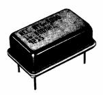
The common thread running through the NTC-4000 TCXO family is its use of our custom bipolar three segment compensation IC. In addition to the IC and the crystal, these oscillators have adjustable thick film resistors for compensation and varactors to provide the changing reactance for temperature compensation. The NTC-4000 Series is available in a hermetically sealed, leaded DIP.
