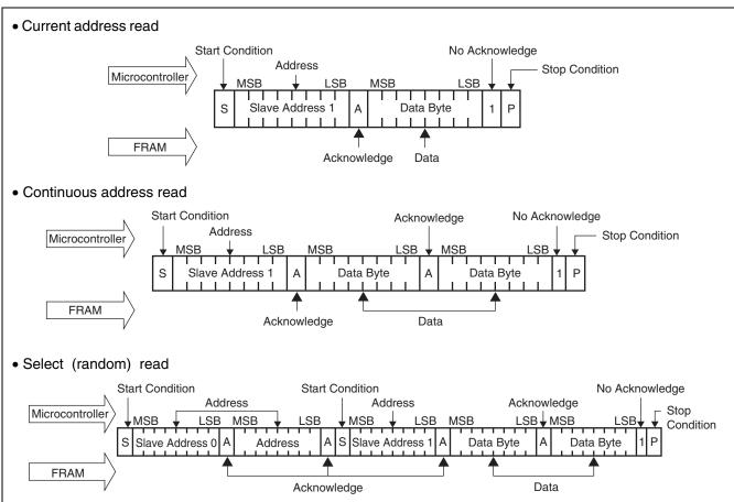
Notes: • When the device is connected to I<sup>2</sup>C external pins (SCL0 and SDA0), the device with the same addresses (1010000<sub>B</sub> to 1010111<sub>B</sub>) as built-in FRAM cannot be used.
