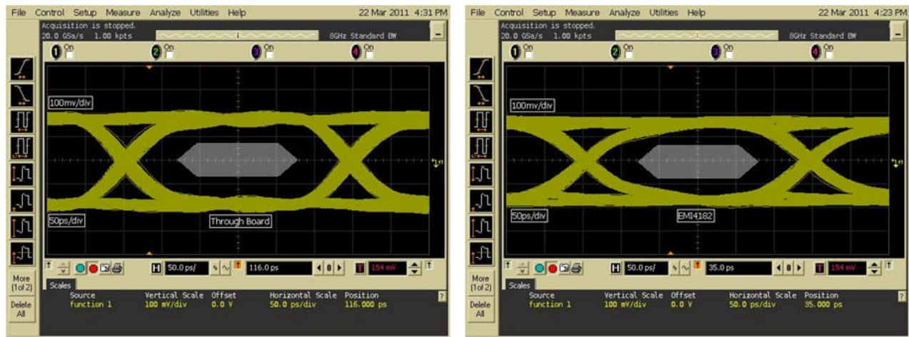
Figure 10. EMI4182 Measured Eye Diagram @ 3.4Gbps (EVB through on left, EVB with EMI4182 on right)
