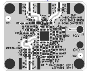
Circuit Board Material: .014" FR-4, 4 layers, .062" total thickness
