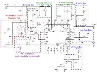
Printed Circuit Board Material: .014" FR-4, 4 layers, .062" total thickness
