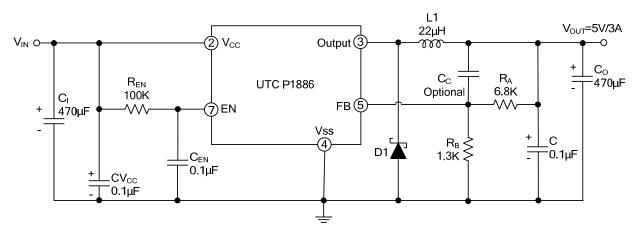
Note:  $V_{OUT} = V_{FB} x (1+R_A/R_B)$ ,  $R_B=0.7K^{\sim}5K$  ohm
