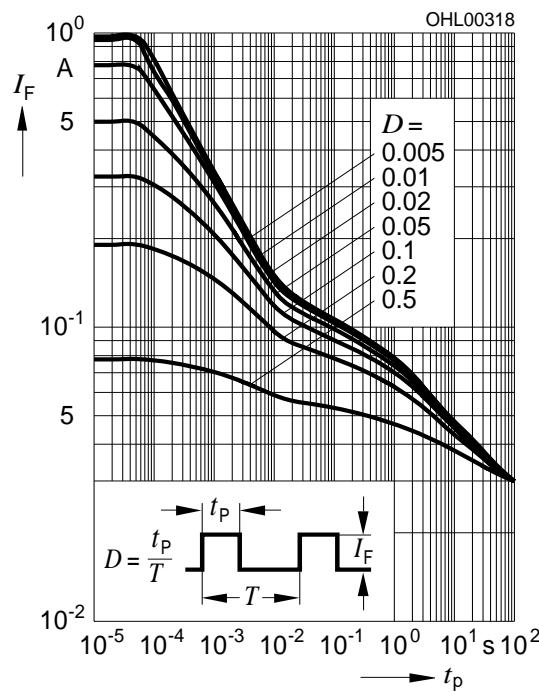
**Zulässige Impulsbelastbarkeit  $I_F = f(t_p)$** **Permissible Pulse Handling Capability**Duty cycle  $D$  = parameter,  $T_A = 85^\circ\text{C}$
