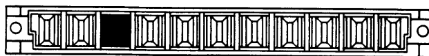
Polarizing Key HCOMK installed in Type H11 female connector — The removal of the corresponding male terminal is required.
