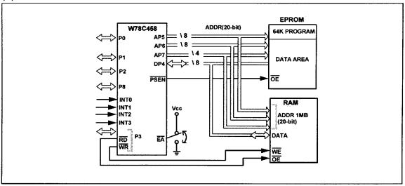
When the EPMA.7 is "1," AP7<3:0> are the output pins to support memory-mapped peripheral chip select logic, which eliminates the need for glue logic. These pins are decoded by AP6<7:6>. Only one of them is active low at any time. That is, they are active individually with 16K address resolution. For
