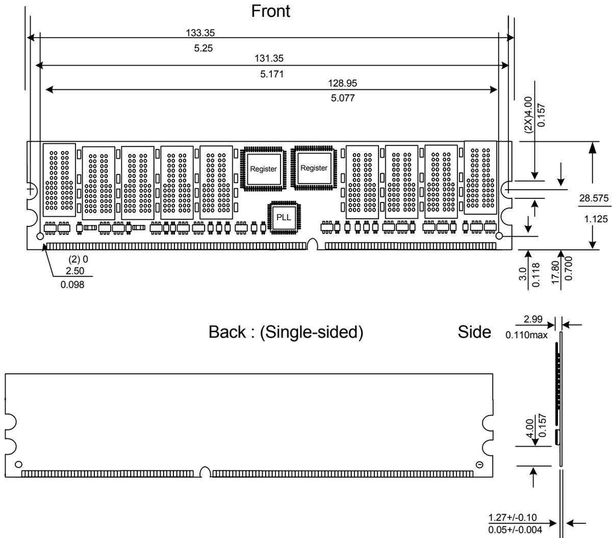
Note) All dimension are typical unless otherwise stated.  $\frac{\text{Millimeters}}{\text{Inches}}$
