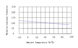
Luminous Intensity Vs. Ambient Temperature
