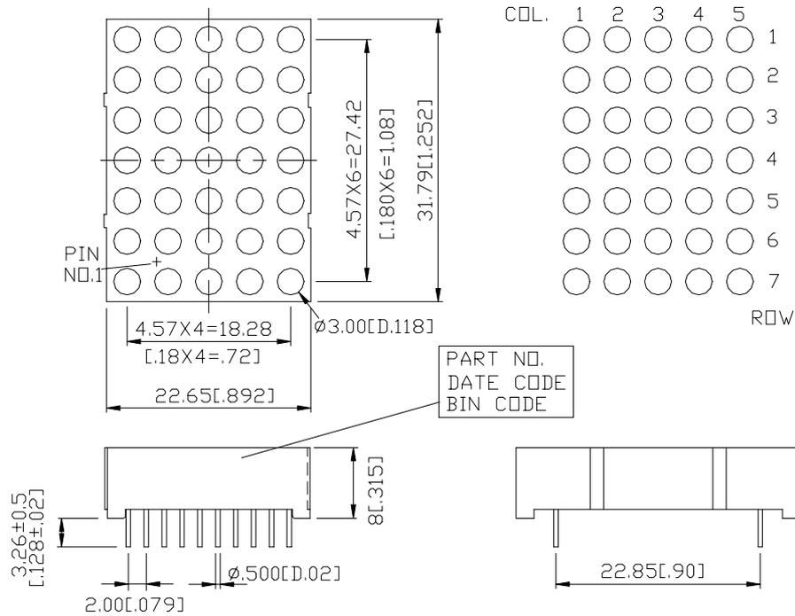
NOTES: All dimensions are in millimeters. Tolerances are ± 0.25 mm (0.01“) unless otherwise noted.
