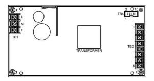
TB2 PIN Assignments: TB2 terminal block connections are for the output Voltage and current and are defined as follows:
