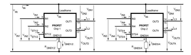
Leadframe (V<sub>bb</sub>) is connected to pin 1,10,11,20
