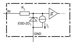
The use of ESD zener diodes as voltage clamp at DC conditions is not recommended.
