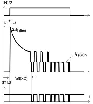
ST1 and ST2 have to be configured as a 'Wired OR' function ST1/2 with a single pull-up resistor.
