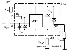
$V_{Z1}$  = 6.1 V typ.,  $V_{Z2}$  = 47 V typ.,  $R_{GND}$  = 150 Ω,  $R_{ST}$ = 15 kΩ,  $R_{I}$ = 4.0 kΩ typ.
