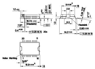
1) Does not include plastic or metal protrusion of 0.15 max. per side
