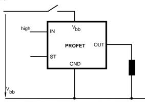
For inductive load currents up to the limits defined by  $Z_L$  (max. ratings and diagram on page 10) each switch is protected against loss of  $V_{\mbox{bb}}$ .
