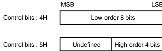
Fig. 2-3 Lock Address Format
