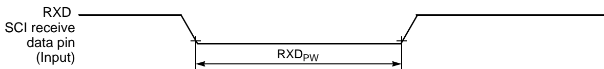
Figure 10-15 RXD Pulse Width
