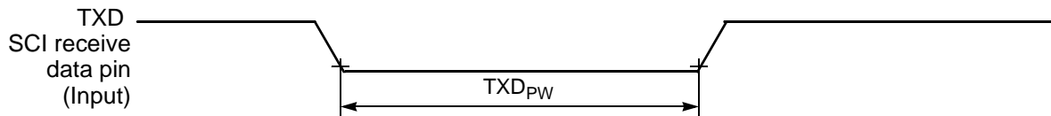
Figure 10-16 TXD Pulse Width
