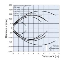
Retro-reflective Models (radial) E3F2-R2R□41-□ (polarizing) and reflectors
