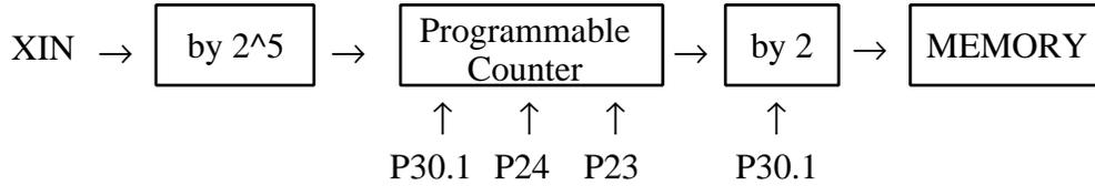
The melody generator consists of a  $XIN/2^5$  clock source (if  $XIN = 3.58$  MHz, the clock source is 112 KHz) and a 8-stage programmable binary counter. The internal ports P23 and P24 control low-nibble and high-nibble of the counter respectively. The contents of P23 and P24 will be loaded into programmable counter automatically when OUTA P23 or OUTM P23 instruction is executed. Bit 1 of P30 controls ON/OFF of melody generator.
