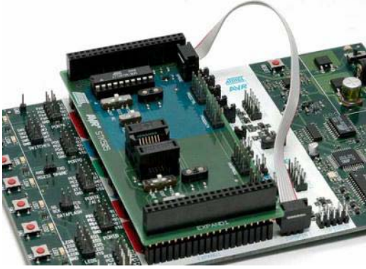
Figure 2-2: In-System Programming of the ATtiny26
