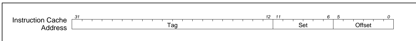
Figure 5-9. Instruction-cache address partitioning.
