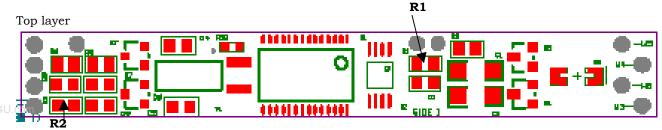
The R2 'pack thermistor' or 'T-pin' signal is used by external devices, such as chargers, to determine the chemistry of the battery pack or it's temperature (using and external circuit.) The P3 module includes this 'T-pin' value at R2 as one of two values. As shown in the parts list, this may be either a NTC thermistor (same as R1) for NiMH applications or it may be a 365 ohm resistor for Li Ion applications.
