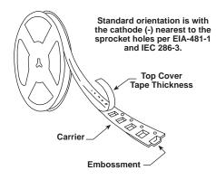
**Tape and Reel Specifications**: All case codes are available on plastic embossed tape per EIA-481-1. Tape reeling per IEC 286-3 is also available. Standard reel diameter is 13" [330mm]. 7" [178mm] reels are available.
