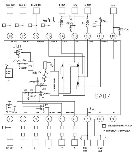
Figure 1 shows the schematic of the evaluation kit's pre-wired connections Components supplied with the kit are marked with an asterisk (\*). All other connections are made via the bread-boarding areas of the circuit board.
