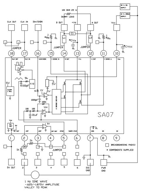
Figure 2 shows a suggested simple test circuit that you can build to gain a familiarity with the evaluation kit as well as the amplifier. At the A OUT or B OUT pads relative to power ground you should observe a square wave with a frequency of approximately 500kHz, 30V p-p which is being modulated from approximately 0 to 100 % duty cycle at a rate of 1 Hz.
