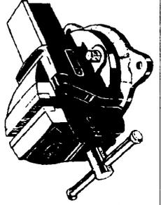
360 degree Swivel Bases rotate & lock the vice at the best working angle. They are available on all but the No. 0 & 2 as standard fittings or optional extras.
