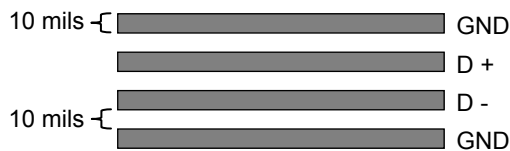
Figure 11. Recommended Remote Diode Circuit Board Interconnect
