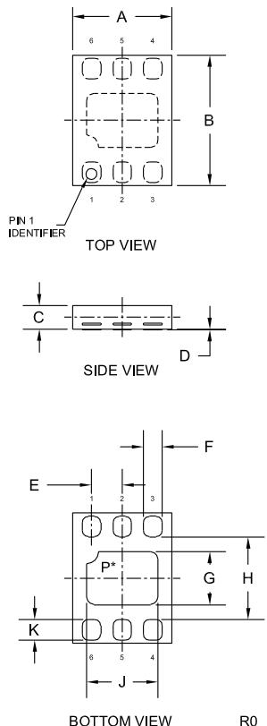
\*Exposed pad P internally connected to pins 2, 3, 4, and 5.
