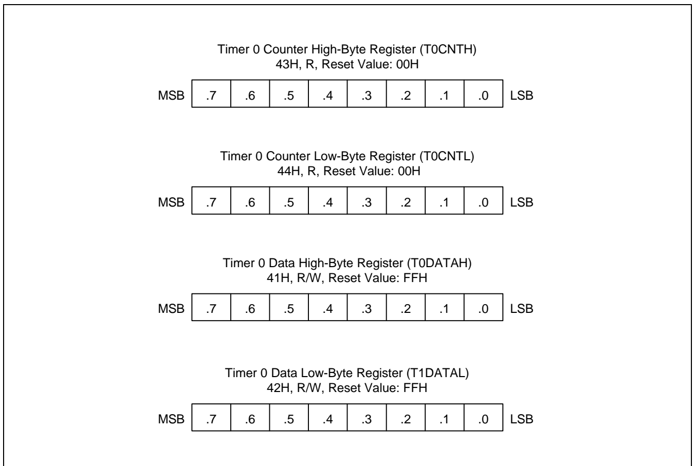
Figure 13-3. Timer 0 Counter and Data Registers (T0CNTH/L, T0DATAH/L)
