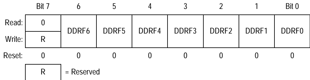
Figure 20-18. Data Direction Register F (DDRF)
