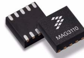
10 PIN DFN 2 mm x 2 mm x 0.85 mm CASE 2154
