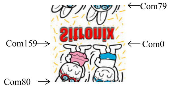
Figure 8.1.1 Common scan direction configuration
