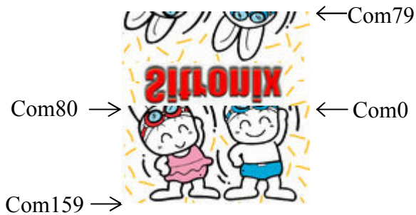
Figure 8.1.1 Common scan direction configuration
