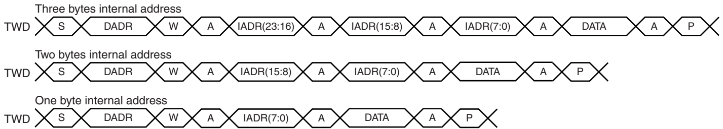
Figure 35-11. Master Write with One, Two or Three Bytes Internal Address and One Data Byte
